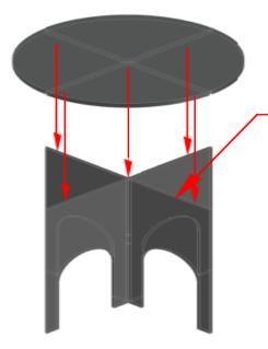
Apply PVC pipe cement to the top. Attach the top and set upside down until the pipe cement is dry. Place in can.
