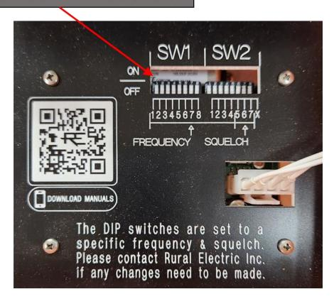
Figure 8 DIP Switch Locations (Frequency & Squelch)
