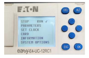
The top line on the screen will flash, and you can see that the controller is in "RUN" mode
