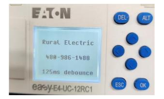
Press the "ESC" button to back out of the menu and return to the main screen. This will password lock your controller. If any other changes need to be made you will need to unlock the controller again
