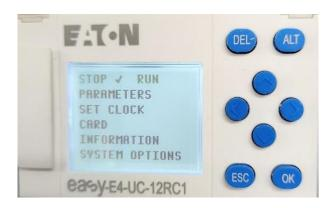
Press to scroll back up to the stop/run options line and press "OK". Select "YES" and press "OK" to return the controller to "RUN" mode
