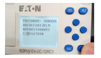
Scroll back up to the top line that says "Password" and press "OK" anywhere on the line. This will return you to the menu screen and your controller will be unlocked for editing
