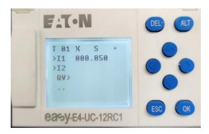
Press the button to scroll over to the desired number and press or to change the number. Scroll over to the next number to repeat the process
