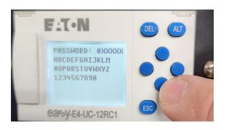
Press the vertice button 3 times to scroll down to the numbers for entering the password
