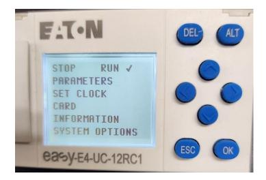
Scroll back up to the stop/run options line and press "OK"
