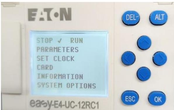
Press ▲ to scroll back up to the stop/run options line and press “OK”. Select “YES” and press “OK” to return the controller to “RUN” mode
