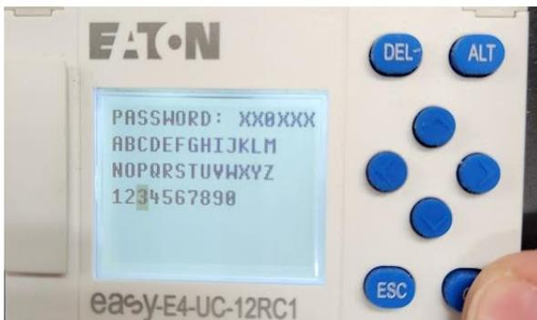
Scroll back up to the top line that says "Password" and press "OK" anywhere on the line. This will return you to the menu screen and your controller will be unlocked for editing
