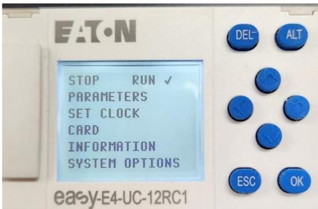
The top line on the screen will flash, and you can see that the controller is in "RUN" mode
