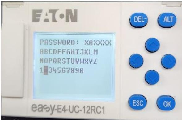
The default password is 1 2 3 4 5 6. Scroll to number 1 and press "OK" to enter it. Scroll over to number 2 using the ► button and press "OK" to enter it. Repeat this process until you have entered all 6 digits
