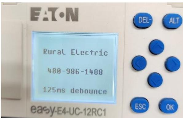
Press the “ESC” button to back out of the menu and return to the main screen. This will password lock your controller. If any other changes need to be made you will need to unlock the controller again
