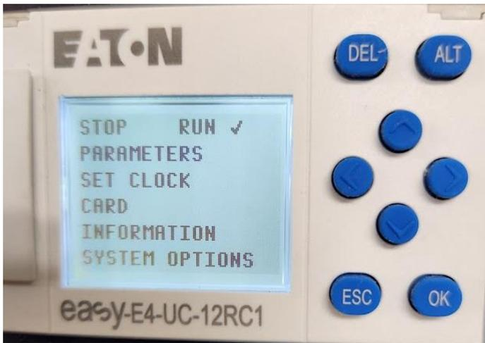
Scroll back up to the stop/run options line and press "OK"
