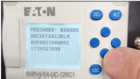
Press the ▼ button 3 times to scroll down to the numbers for entering the password
