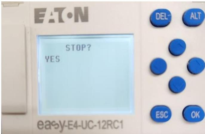
Select "YES" and press "OK" to put the controller in "STOP" mode. This allows settings to be changed
